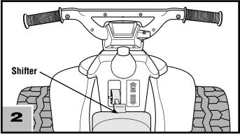
IMPORTANT! To avoid damaging the motors and gears, make sure to stop the vehicle before switching from forward to reverse.
